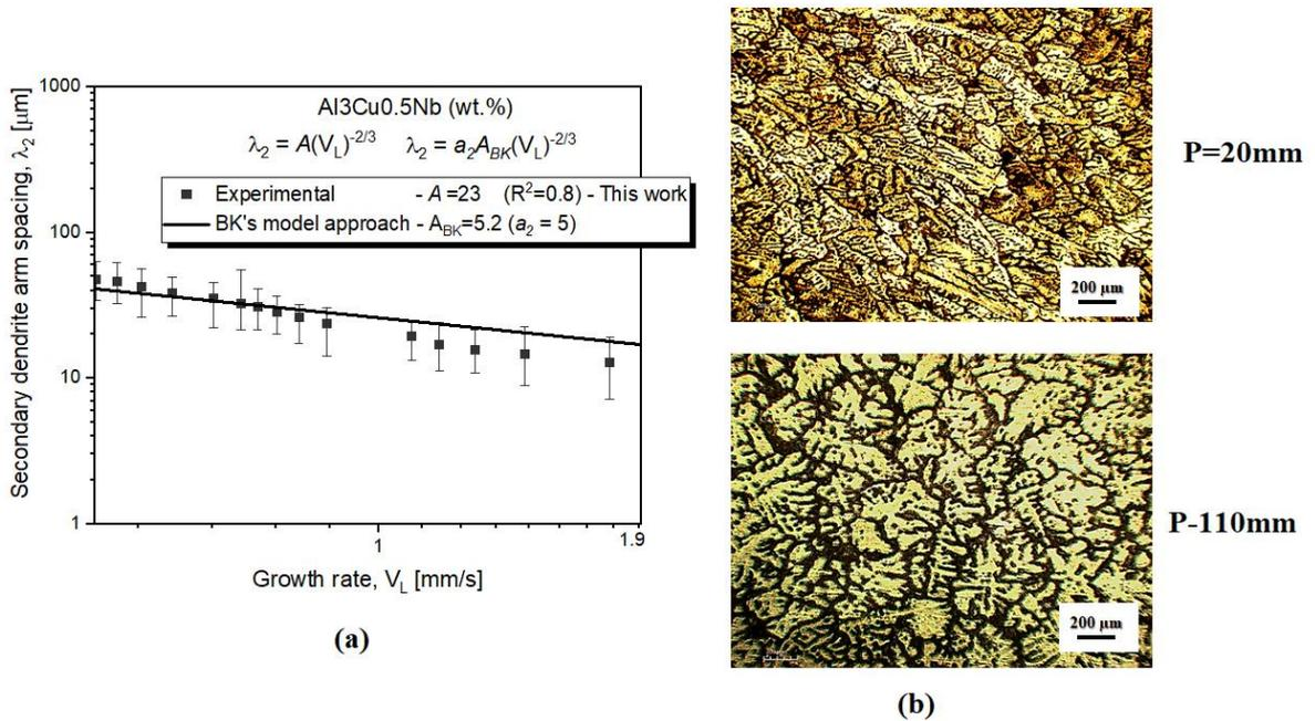
Figure 2. Secondary dendritic spacings: (a) theoretical-experimental analysis, and (b) typical solidification microstructures of the investigated alloy
