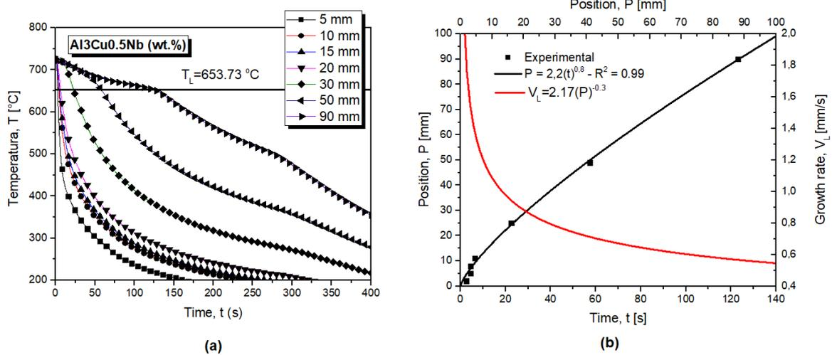
Figure 1. Typical experimental curves of each thermocouple, solidification kinetics, and growth rates for the investigated alloy.
