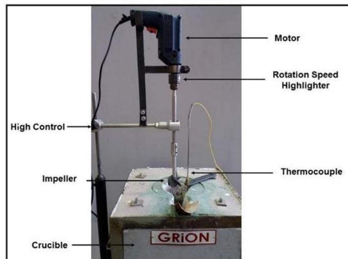
Figure 1: Developed stir casting setup
