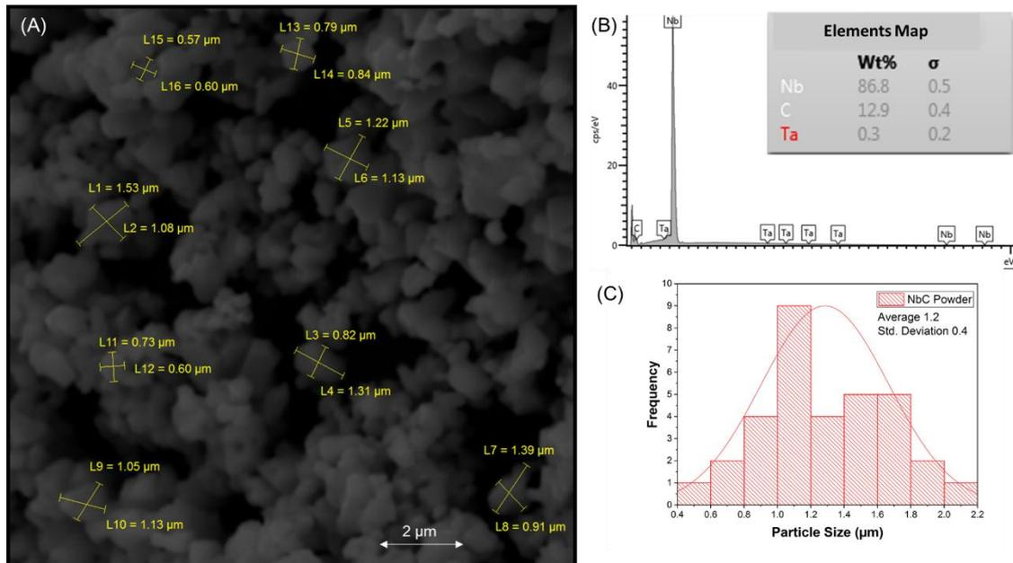
Figure 2: (A) Backscattered electron MEV image from NbC powder respective chemical composition from EDS (B) and particle size from ImageJ analysis (C).
