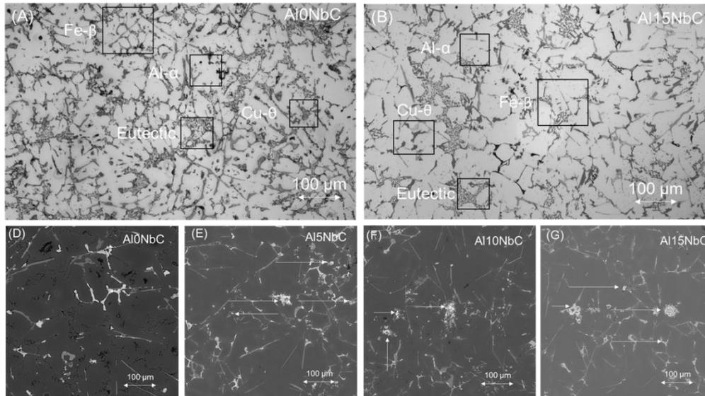
Figure 4: Microstructure of the composites showing the phases (A) Al0NbC (B) Al15NbC, BSE MEV images showing the NbC particles, denoted by white arrows Al0NbC (D), Al5NbC (E), Al10NbC (F) and Al15NbC (G).
