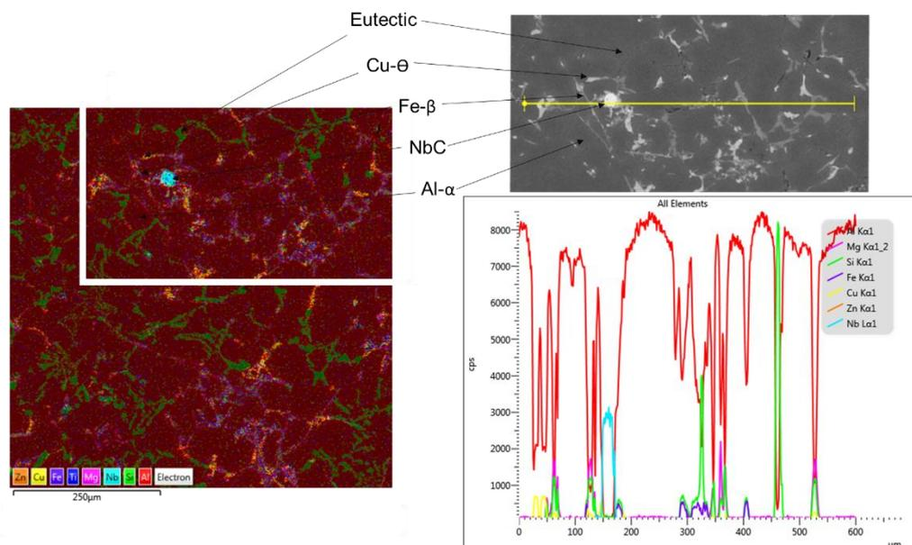
Figure 3: EDS map and line scan of Al5NbC composite with marked formations
